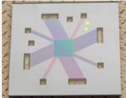
Nanofluidic molecular filter array microdevice for fractionating proteins. Jongyoong Han
