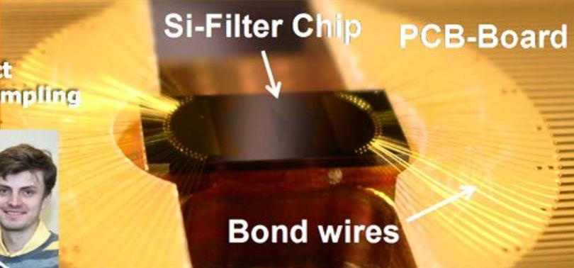
Fig. 1 above: Twenty channel optical demultiplexer consisting of twenty second-order silicon microring-resonator filters with precisely spaced resonant frequencies.
